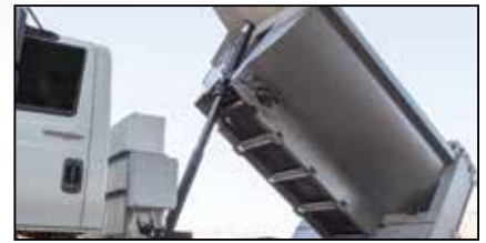
Mailhot® multi-stage, double-acting, nitrified cylinder, trunnion-mounted hoist
