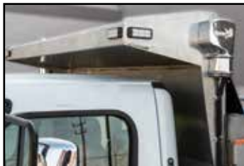
Cab shield with Tarp System
